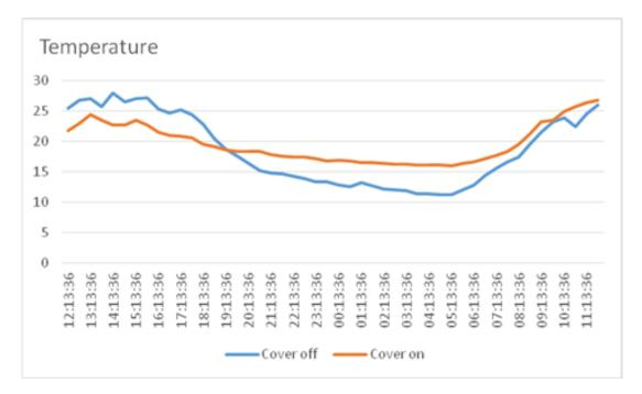
**Figure 5.** Effect of covering *Geum* plants with polythene on temperature (°C) in the plant canopy. Data shown are for the cover on (22 - 23 August, top line) and cover off (20 - 21 August, bottom line) for a 24 h period.
